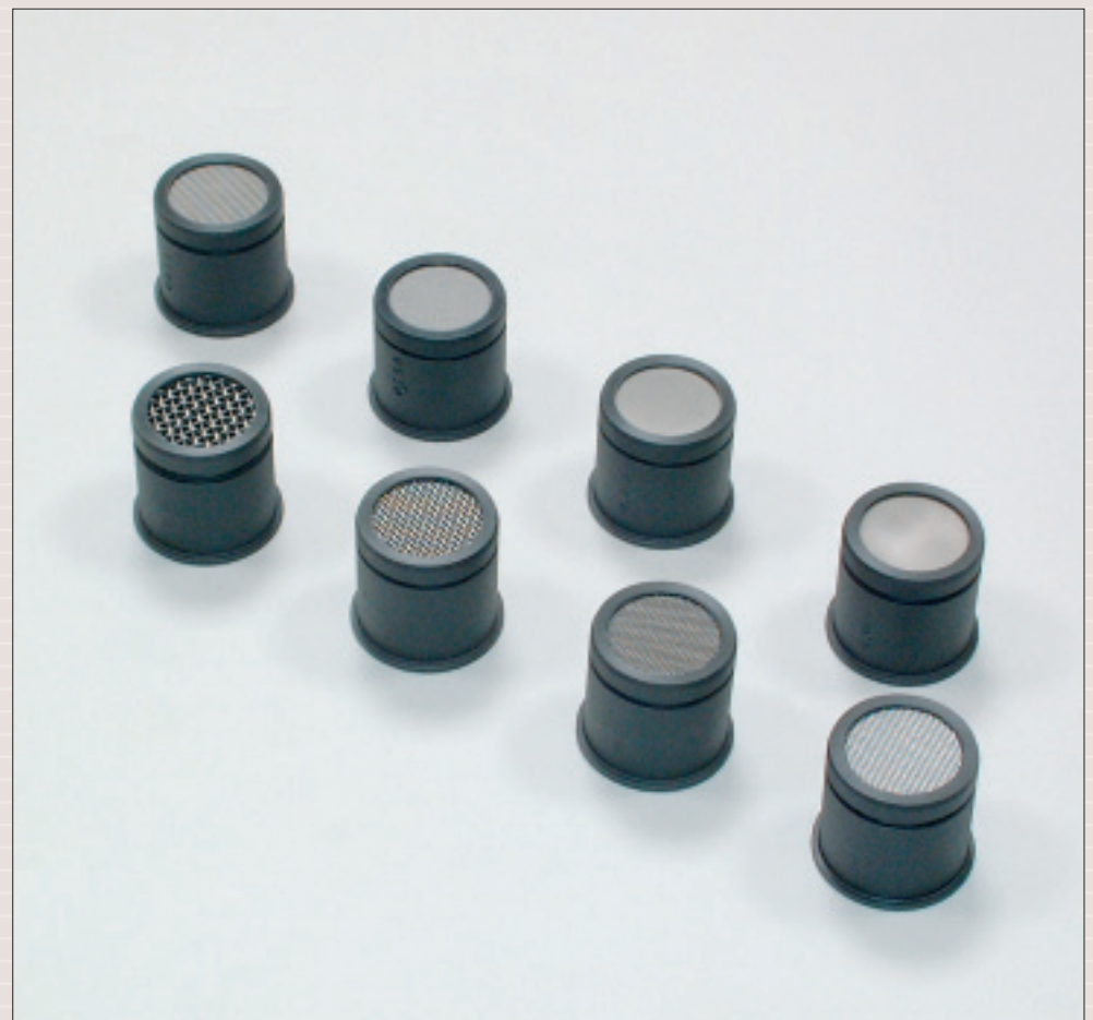
Sieves with openings 2.0 - 0.045 mm.
